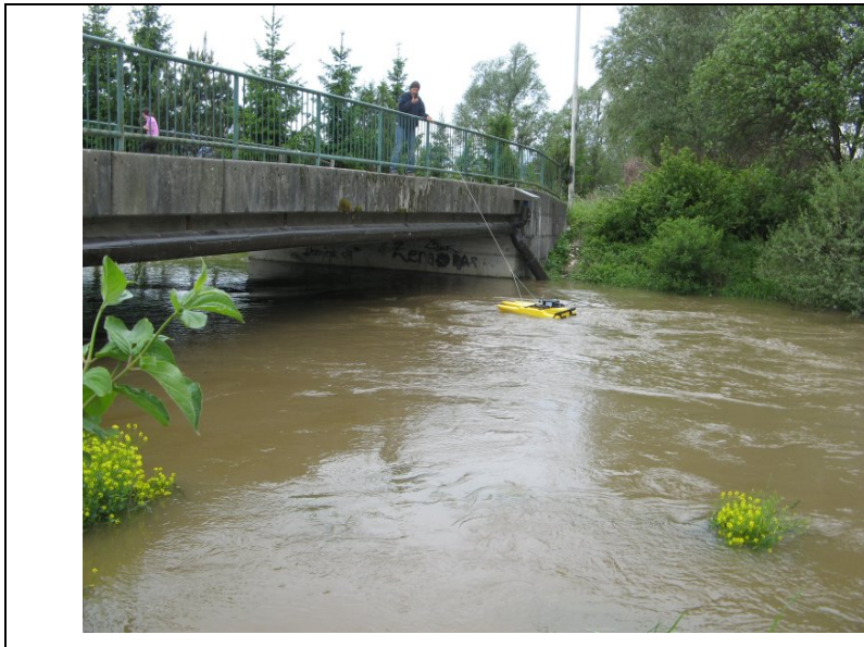
Figure : Ultrasonic Doppler flow measurement, periodic field measurement during high water, 28.10.2012
