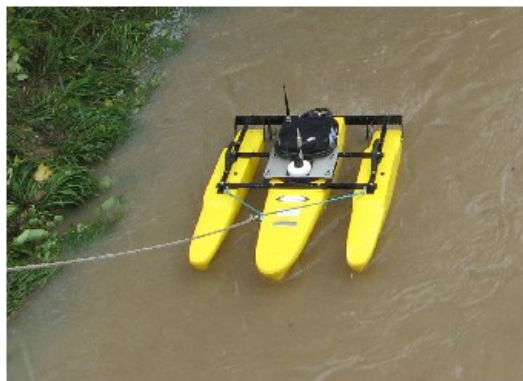
Figure 14: The ADP measurement device - measuring the high water flow in Ljubljanica River
