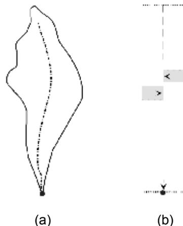
Figure 1.: Simple watershed with kinematic-wave model representation
