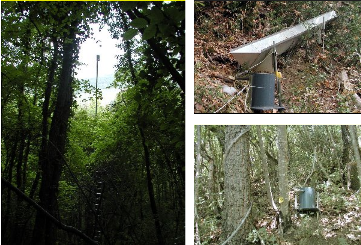
Figure 2. Precipitation measurements above the canopy (left), throughfall measurements (right, above) and stemflow measurements (right, below).
