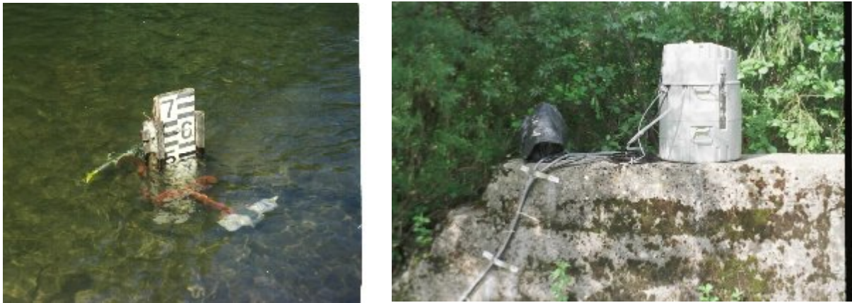
Figure 6. Valeport self recording current meter and Starflow ultrasonic velocity meter (left), and ISCO 6700 compatible area-velocity module (right).
