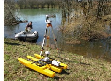
Figure 11: Performing discharge measurements in Planina
